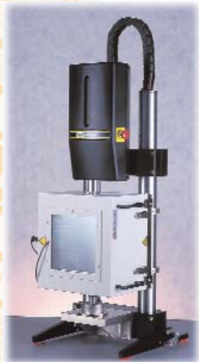
► Temperature humidity chamber mounted on a vertical MicroTester
