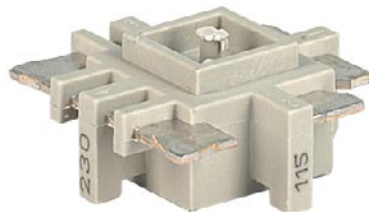
Figure 6. Voltage selector unit
