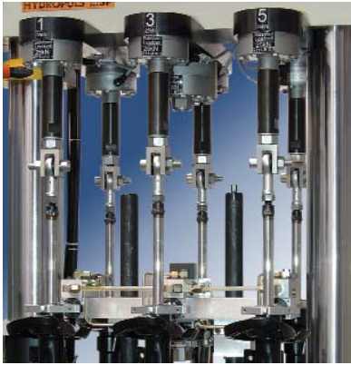
▲ Side load input for six dampers
