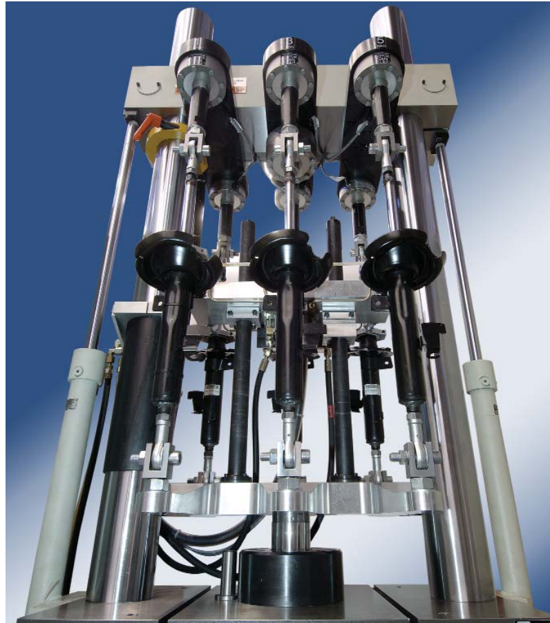
▲ MSP test system for testing six shock absorbers
