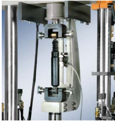
▲ Side load input into a single damper
