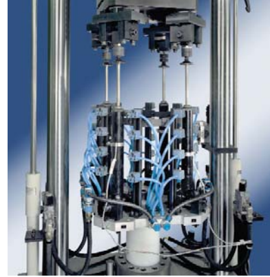
▲ Side load input into four dampers. System includes air cooling
