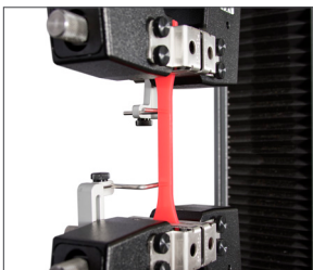
Specimen Alignment Device helps to get the best repeatability from your system.
