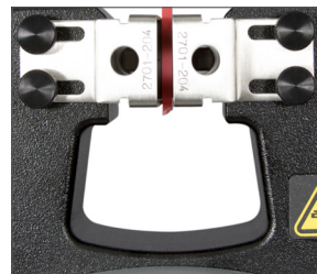
Large throat size allows for easy specimen insertion.
