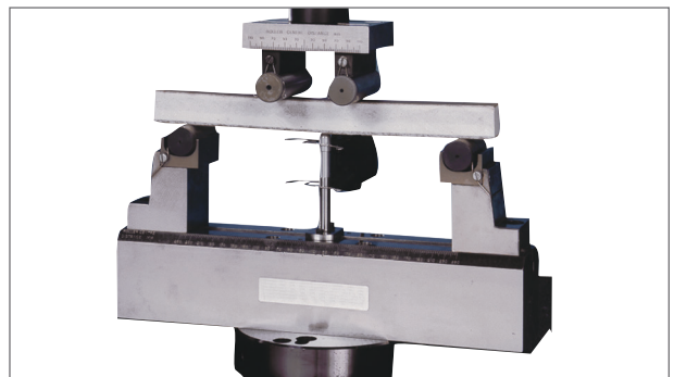
Four-point loading using mid point deflectometer
