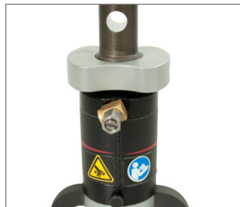
Airflow Adjustment valve on 50 N grip
