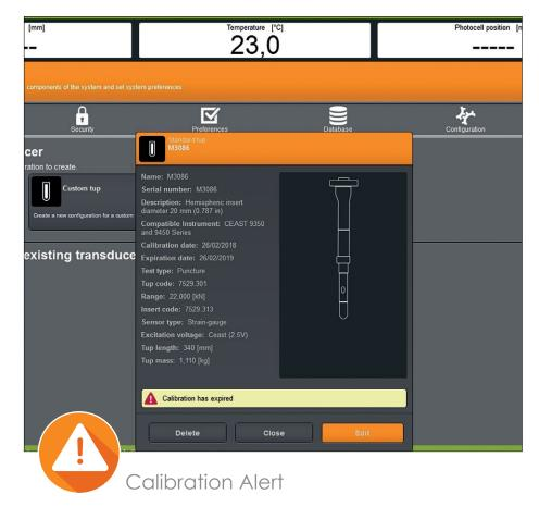
Automatic alerts are generated when Tup calibration period is expiring. This feature helps to reduce the risk of invalid tests and protect your results against inaccuracies.
