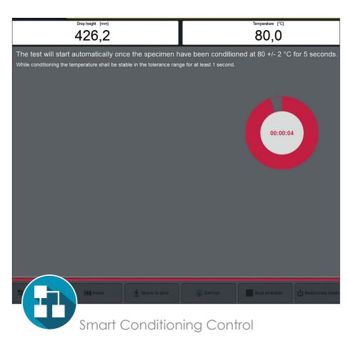
Bluehill Impact is able to control temperature stabilization within the thermostatic chamber.
