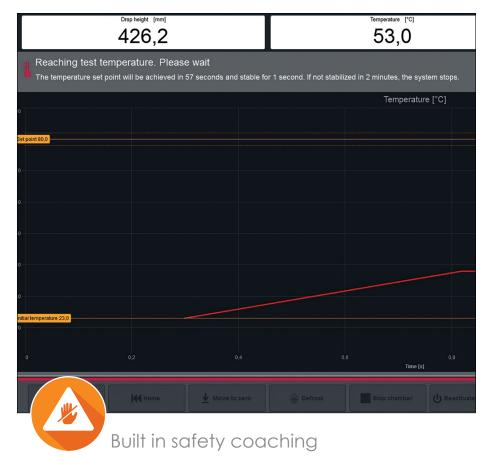
The 9400 system is a fully enclosed system to conform with CE regulations. As an additional safety measure, the system gives clear visual information on the instrument status, so users always know when a test is in progress. Bluehill Impact security allows the Lab manager to configure permissions in the software, granting full permissions to super users and limiting access where needed.
