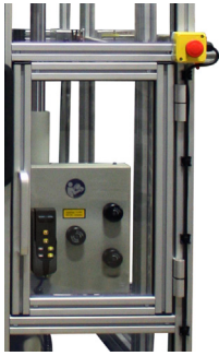
Interlocked Safety Enclosure which restricts access to the test area during test
