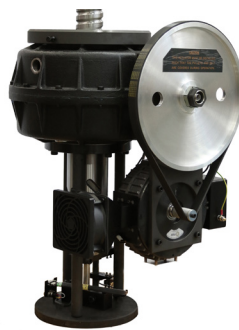
Backlash free servo-electric actuator option for low strain rate specifically designed testing
