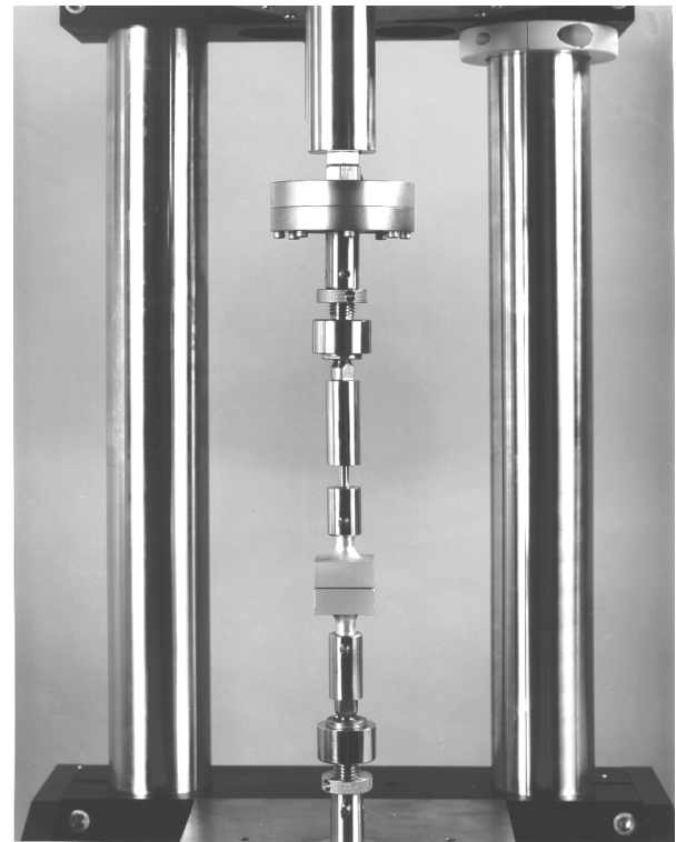
Figure 3 - Stud Pull Fixture Mounted in a Testing Machine
