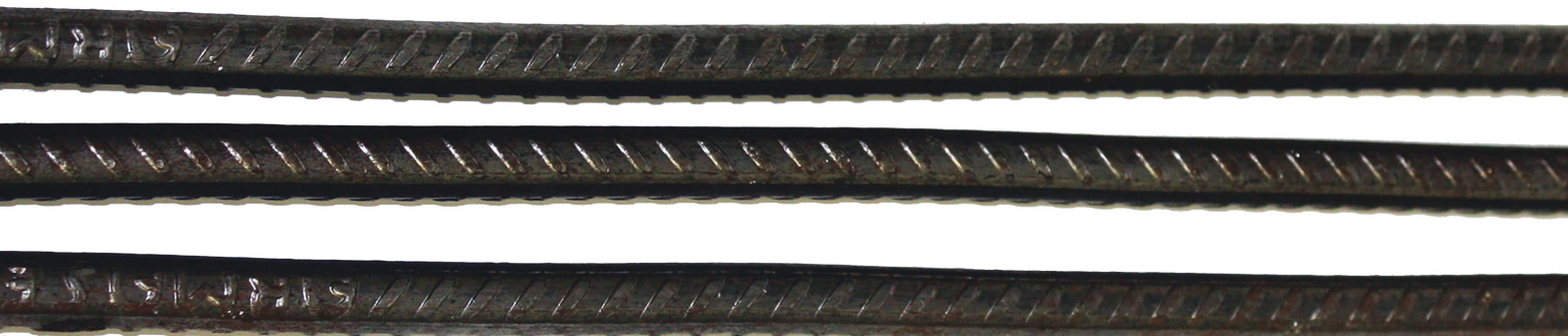
Uncoiled rebar with slight bends over length.
