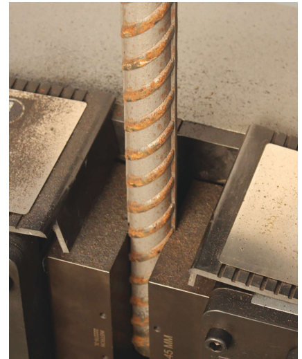
Abundant scale accumulation on lower grip after one test.
