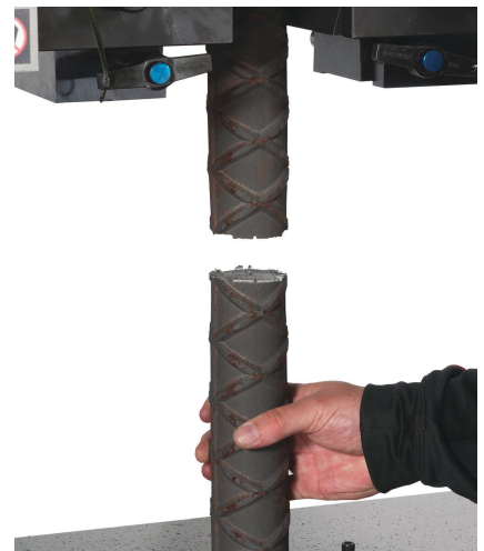
Number 18 (57 mm) bar separation (recoil) after failure.
